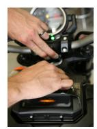
5. Keep both mode switches depressed until "15" appears where "DIAG" previously appeared. This is your bikes Diagnostics screen. 3. Keep both mode switches depressed until "DIAG" is shown in the upper left corner of the Meter 2 display.
