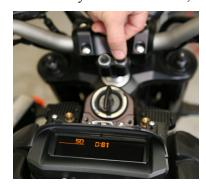
9. Cycle the Run/Stop switch and all fails should clear. If D:62 indicates "0", there are no faults. Turn the Key switch off. Reset complete.
