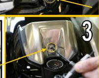
3&4:Remove Meter 2 Visor and Top Screws: Using a 4MM Allen, remove the screw securing the metal sun visor over Meter 2 display. Once the sunshade is removed, you will have access to the 4 screws that secure the Faux tank Cover to the Main Switch Housing and Meter 2 mounting screws.
