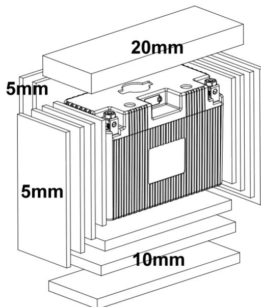
The LFX batteries can bolt cable eyelets to either the top or front sides of the terminals. Choose whichever allows best cable fit. Max torque for the terminal screws is 4.5kg/cm (60 oz/inch). Do not over-tighten. A quality anti-corrosion spray is recommended for the terminals, and required if used in salty and/or wet environments. Battery failure due to terminal corrosion is not covered under warranty.
