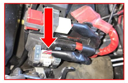
Find the Switched Supply wire that is located on the left side of the battery box just below the Main 30A fuse. Locate the Red Wires with White Stripes. There are two. Either is acceptable for tapping.
