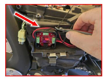
After installing all of your additional circuits and testing them, it will be time to tidy the wires and install the lid. Bundle the wires tightly to the top of the Buddy Box and use the included Zip Ties to secure them in place.
