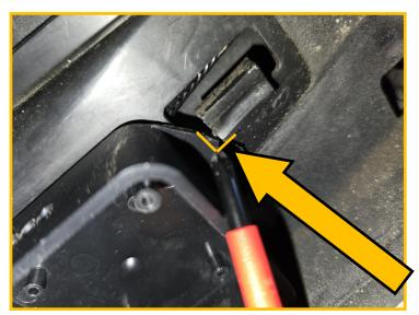
Install the Fuse Buddy Box Base in the now empty upper section of the Left Side Cover. You will have to slightly trim the Buddy Box tab. This can be done by touching it to a grinder wheel or trim it with some side cutters for it to fit properly. You will make a very small notch in the tab to accomplish this.
