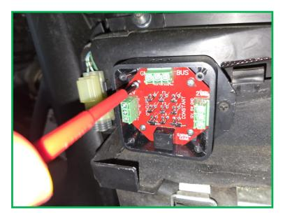
Now insert the PCB board with the small black cubed relay at the bottom and the board to the Buddy Box using the 4 stainless Phillips screws.
